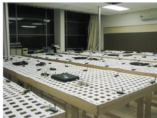
Figure 11: *NetEye* wireless sensor network testbed
